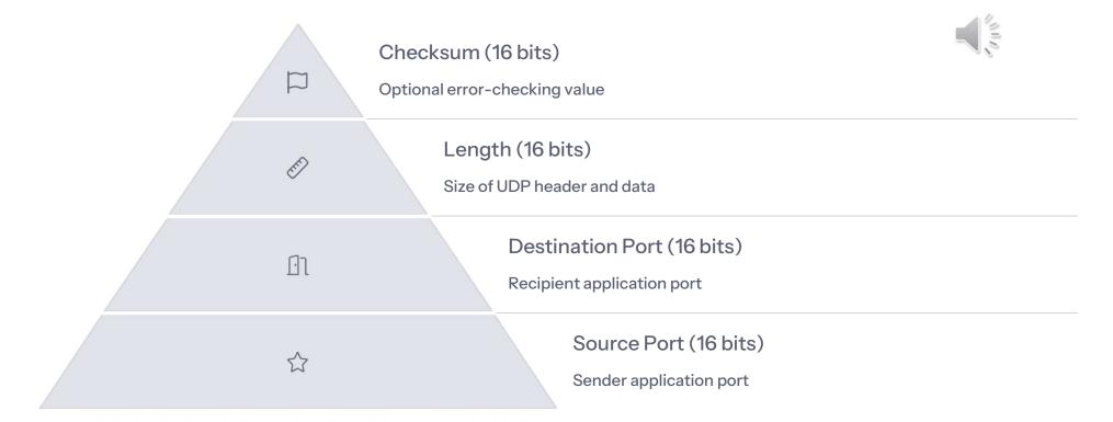
The UDP header is remarkably simple with just four fields totaling 8 bytes. This minimalist design contributes to UDP's low overhead and fast transmission capabilities. After the header comes the actual data payload, which can vary in size up to a practical limit determined by the underlying network.
