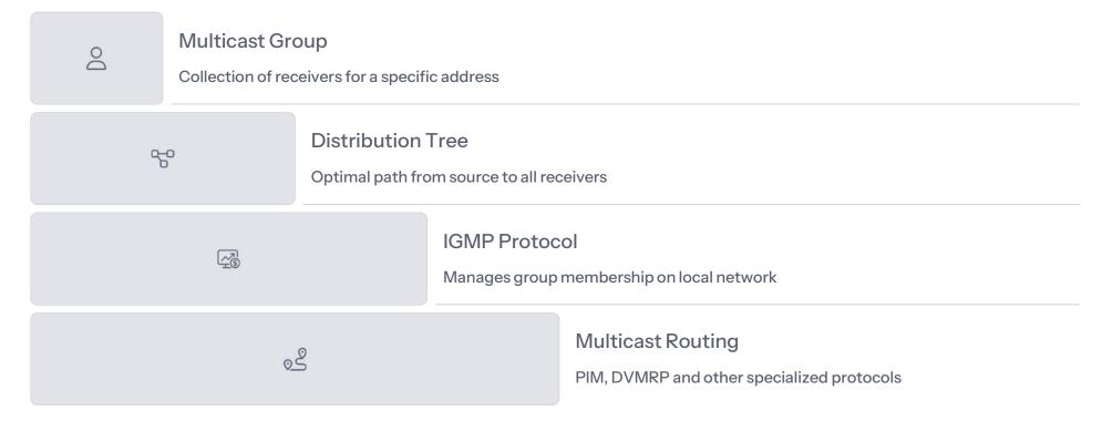
Multicast relies on specialized network infrastructure to work efficiently. Hosts use IGMP (Internet Group Management Protocol) to signal their interest in joining or leaving multicast groups. Multicast-enabled routers use protocols like PIM (Protocol Independent Multicast) to build distribution trees that efficiently deliver packets to all group members.
