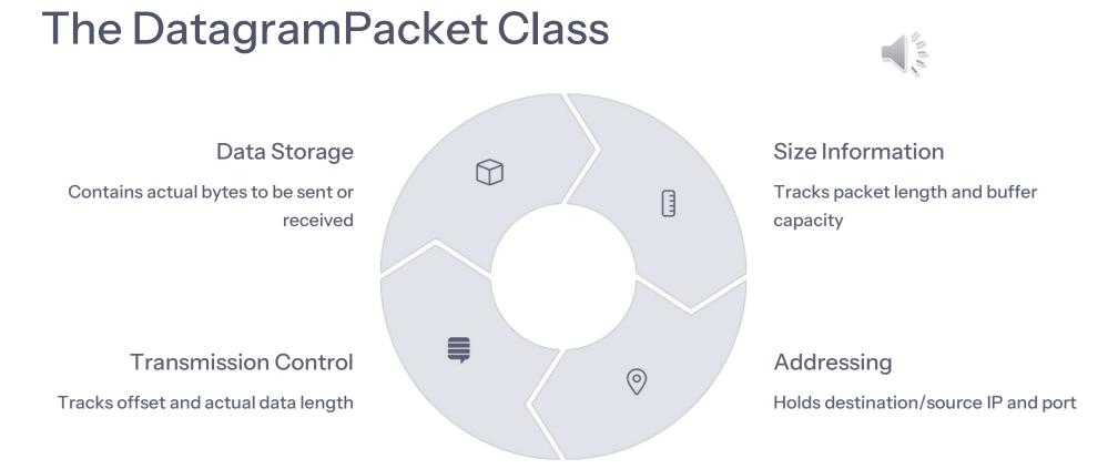
The DatagramPacket class serves as the container for UDP data transmission. When sending, it encapsulates the message data along with destination information. When receiving, it provides buffer space for incoming data and captures the sender's address information for potential responses.
