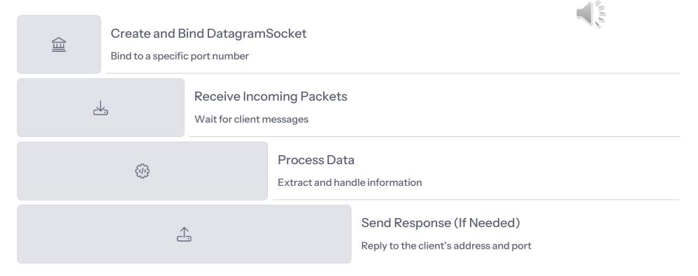
UDP servers operate differently from TCP servers, as they don't maintain connection state with clients. Each packet is processed independently, and the server must extract the client's address and port from the received packet to send any response back to the correct destination.
